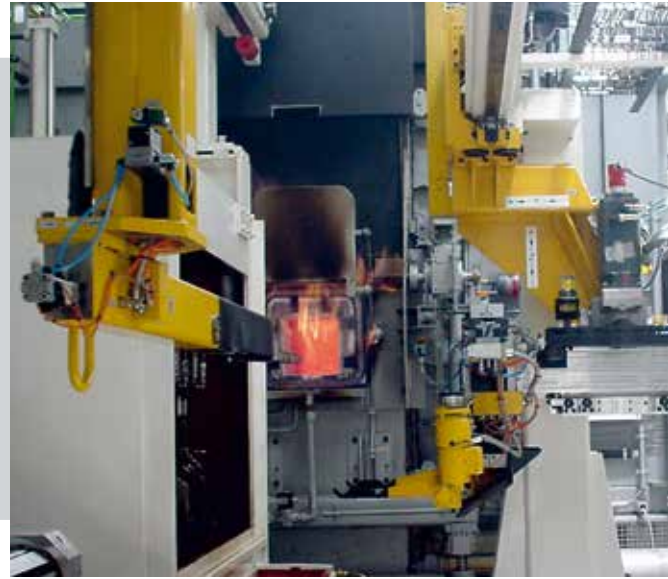
Carburizing and rotary hardening of shafts.
