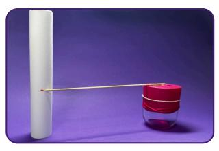
Set up your new barometer and the paper column in a place where they can stay for several days. Mark the height of the pointer and the current weather on the paper column.
