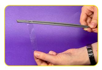
Take two to three sparklers. Leave the top 5 mm free and wrap adhesive tape (approx. 3 cm long) around the following part of the sparklers.
