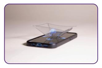
6 Set the brightness on your smartphone to maximum and place the pyramid upside down (with the smaller opening facing downwards) on your screen. Darken the room as much as possible. Start the video and watch the objects float.
