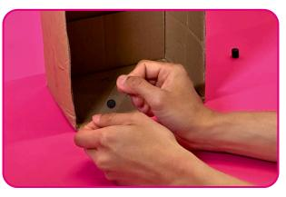
4 Glue the magnets in equal distance (~l-2cm) to one another directly below the resting position of the paper clip.
