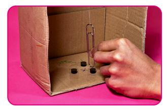
Adjust the string so that the paper clip is attracted by one of the magnets, yet not be able to touch it. Make sure that if the paper clip is released near any magnet it is able to stay on top of that magnet by magnetic attraction.
