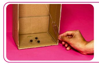
Release the paper clip pendulum from somewhere far from the magnets. Observe its motion. Try to release the pendulum again and again from the same starting position and observe.
