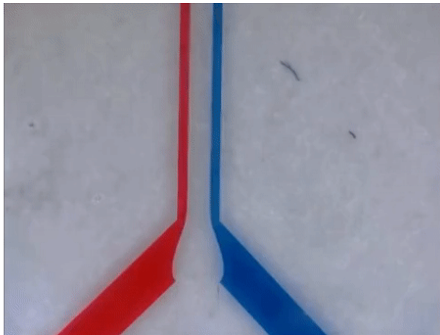
Figure 1. Laminar flow in microfluidics
