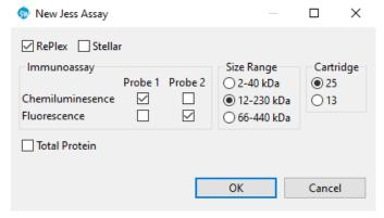
To run one immunoassay and one Total Protein assay - Select Total Protein, then select any combination of chemiluminescence or fluorescence for Probe 1. Probe 2 will be used for the Total Protein assay. For example:
