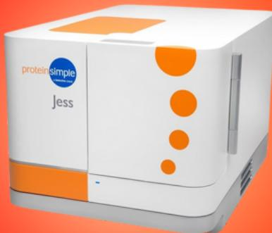
Jess is a fully automated, capillary-based Western blot system that performs immunoassays with high sensitivity, speed, and reproducibility. It streamlines the traditional workflow by automating protein separation, antibody incubation, detection, and analysis.
