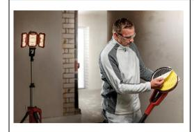
A new sanding concept from scratch: FLEX multihole sandpaper with foam rubber interface pad and Velcro sanding disc with centring aids ensure less vibration and better extraction. (Photo: anw\_ge6r\_10.jpg)
