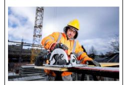
Ready for use on the construction site: The CS 68 18-EC in action – lightweight, robust and ergonomic, with sophisticated features such as LED light, rafter hook and dust extraction.
