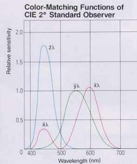
The Yxy color system was defined by the CIE (Commission Internationale de l'Eclairage) in 1931, and forms the base for other CIE color systems. In this system, Y is the lightness factor expressed as a percentage based on a perfect reflectance of 100%; x and y are the chromaticity coordinates in the CIE x, y chromaticity diagram (shown at left), and are defined by the following equations:
