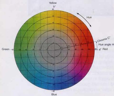
The L\*a\*b\* color system is one of the uniform color spaces recommended by CIE in 1976 as a way of more closely representing perceived color and color difference. In this system, L\* is the lightness factor; a\* and b\* are the chromaticity coordinates. Their defining equations are as follows:
