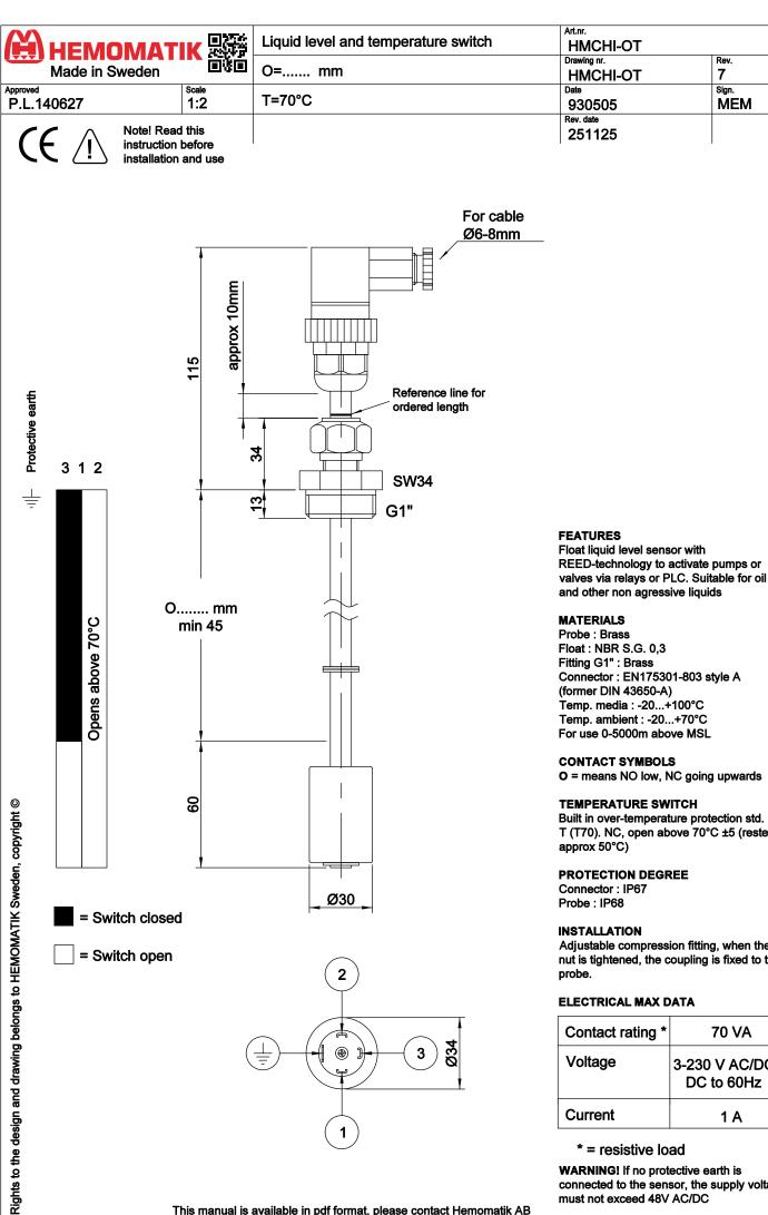
O = means NO low, NC going upwards
