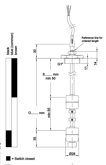
INSTALLATION- Compression fitting Decide and adjust level, once the nut is tightened the compression ring is firm and pressure tight on the stem.
