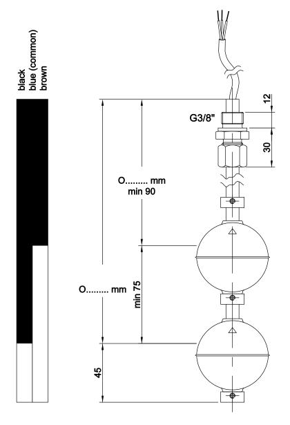
**INSTALLATION-** Compression fitting Decide and adjust level, once the nut is tightened the compression ring is firm and pressure tight on the stem.
