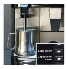
**4.** Submerge steam wand into steaming pitcher and press the LATTE STEAM button to heat solution. After steam wand shuts off automatically then let it soak for 5 minutes.
