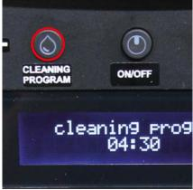
10. Press (do not hold) the blinking  $\Diamond$  button to activate cleaning cycle (this takes about 4:30 minutes). All beverage selection buttons will be locked during this time. Cleaning runs (4:33 min.)
