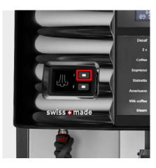
**14.** After wiping off wand, point it toward drip tray and purge by pressing the button 1.
