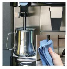
**13.** Submerge steam wand into cold water once to rinse, then discard water. Wipe steam wand with a clean, damp cloth.
