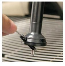
**12.** Using small cleaning brush, brush the 4 side holes as well as base of the steam wand tip.
