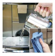
11. After 5 minutes or when automated cleaning cycle is complete, empty pitcher into drip tray. Wipe steam wand with a thick, clean, damp cloth. Be careful, wand will be very hot!
