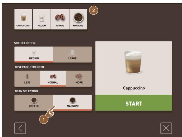
Figure: Frequent user mode: Directly choosing beverage modification
