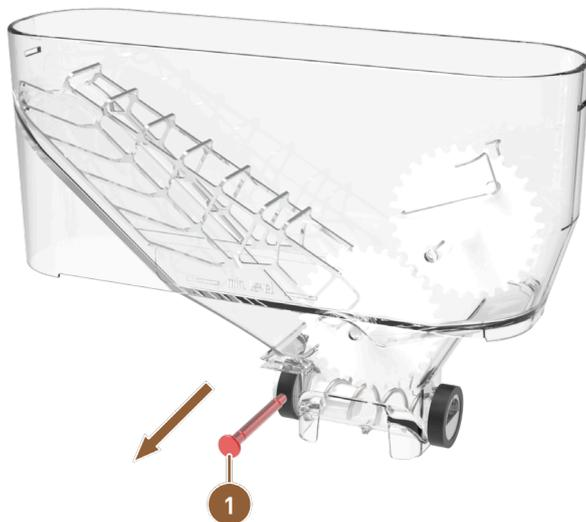
Figure: Standard powder container: Removing lower axis
