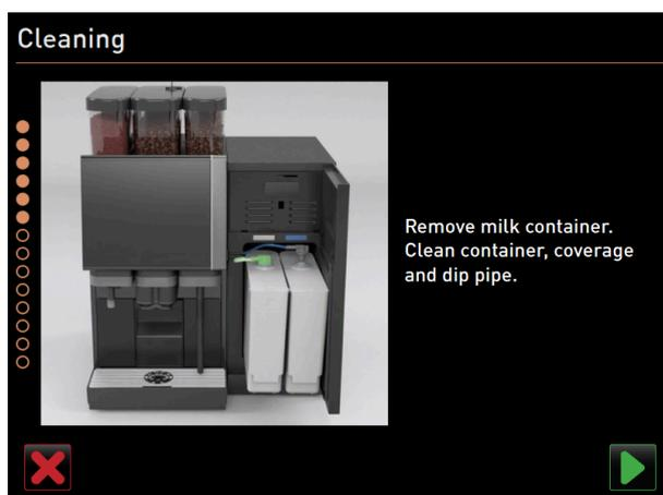
Figure: Cleaning milk container (option)
