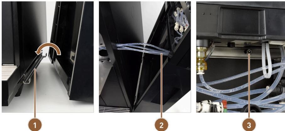
Figure: Fastening ProCare unit to machine
