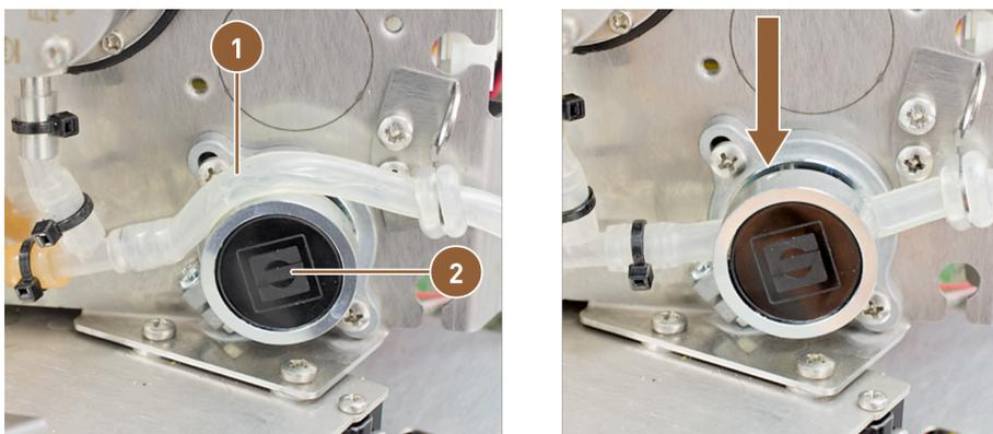
Figure: Inserting milk hose into squeeze valve (Single Milk)
