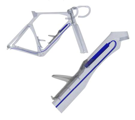
Run the Di2 wires from the front and rear derailleurs to the hole in the downtube, below the bottle cage. Connect the wires to the battery, already fixed to the bottle cage with the specific support, insert into the frame and fix the bottlecage following the steps in section 'Y1Rs Custom bottle cages installation'.
