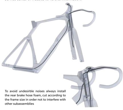
Before to route the brake hoses it is recommendable to install the headset and fork following the Steps 1 and 2 in the dediceted section. Once installed and routed the rear brake hose in the dowtube, with a dedicated wiring tool with magnet in the end, pull the it through the preload bolt hole as shown in the pictures below.
