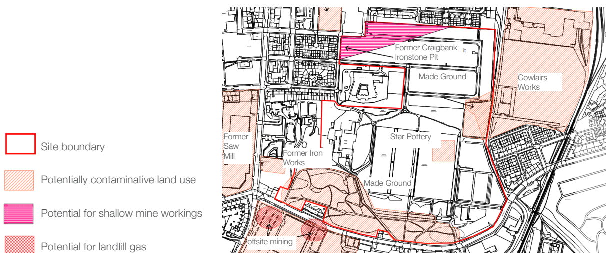
Fig. 3.6 Geotechnical and geoenvironmental hazards. AECOM 2010. Not to scale.
