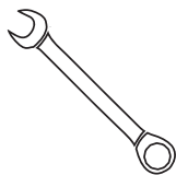
Open-end wrench/ adjustable wrench Tighten or loosen fittings and connections
