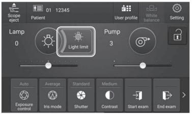
4. After deactivating Light Limit Mode, the icon will disappear from the monitor screen, indicating that the light emission has returned to its normal intensity.
