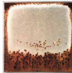
Galvanised steel Z275 (Heavy sign of Rust)
