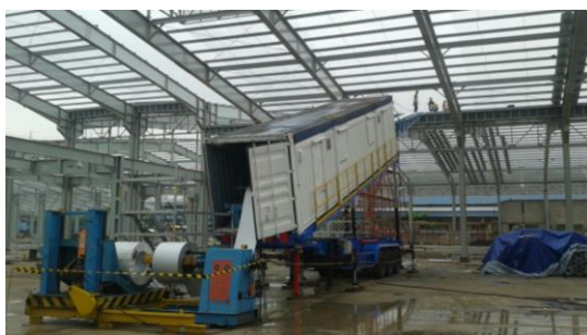
Mobile Elevated Rollforming (MERF)
