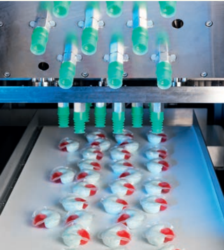
Forming, filling, and sealing of the water-soluble films used for detergent or dish-washing tabs.
