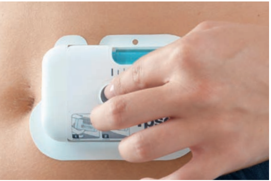
The controlled injection is then triggered at the push of a button.
