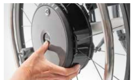
The wheel can be removed by pressing the button on the quick-release axle and pulling the wheel off.
