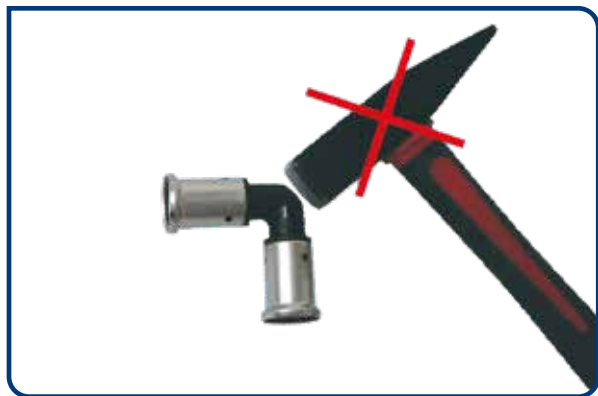
Impact force on PVDF fittings is not allowed.
