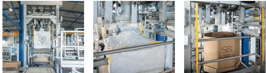
The semi-automatic big bag filling station makes it possible to fill big bags (FIBC - flexible intermediate bulk container) with one, two or four loops and octabins with a filling station of 500 kg to 1500 kg.
