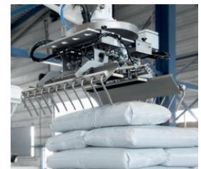
The high-performance robot palletizer PRINCIPAL-R, an articulated arm robot palletizing system, is always offered as a customer-specific solution with renowned industrial robot manufacturers and STATEC BINDER expertise. A special feature of the PRINCIPAL-R is that it was optimized for sling bags.
