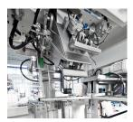
As the name suggests, the FFS-Combi Version of the open-mouth bagging machines has an additional FFS module, allowing bags not only to be used from the bag magazine, but also to be produced from tubular film. The CERTOPAC and PRINCIPAC open-mouth bagging machines are available as FFS-Combi Versions. The additional FFS module is also available for the CIRCUPAC bagging carousel.
