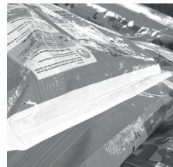
The patented bag sealing system "Over Tape Bag Sealer" from STATEC BINDER heat-seals woven polypropylene (PP) bags airtight. PP fabric tape is used for this purpose to ensure a reliable and secure seal. If necessary, the bags can also be sewn shut. Pillow and gusset bags can both be securely sealed. The sealing technology makes it easier to handle dusty and odor-intensive products in the food and feed industry.
