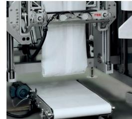
The SYSTEM-F, a fully automatic vertical FFS bagging machine, produces pillow bags and gusset bags from flat film. Moreover, the bags can be made with or without a carrying handle and for a filling weight between 5 kg and 50 kg.
