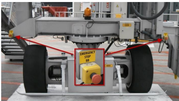
Fig. 48. Locatie externe noodstop boarding bridge pier A
