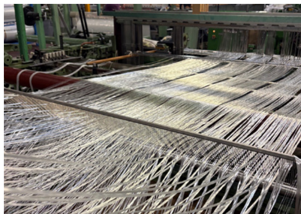
Weaving of recycled glass fiber
