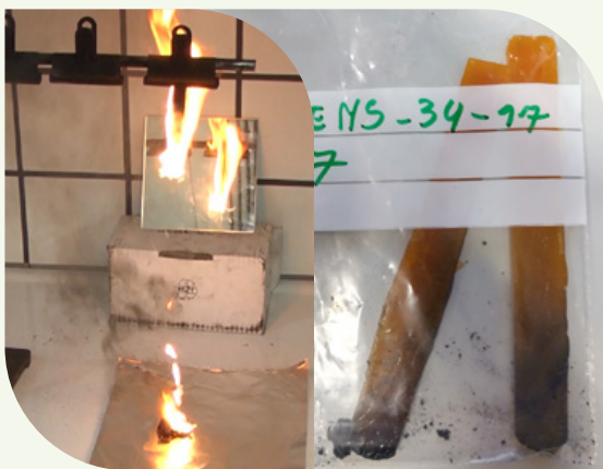
UL94V test without flame retardant (sample completely burnt)
