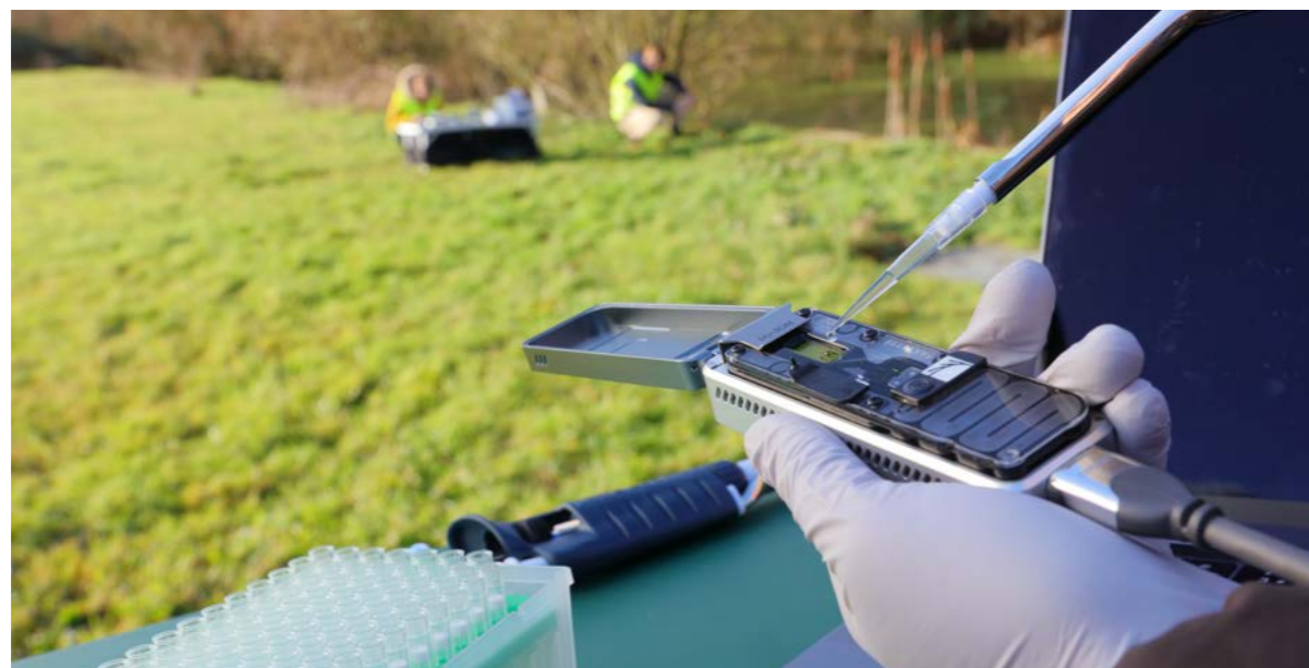
The portability of the Oxford Nanopore MinION Mk1B sequencer means that it can be deployed in a range of settings, with potential to provide rapid, on-site analyses including in the field, for example for environmental or water analysis.
