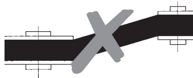
Axial misalignment of sheaves
