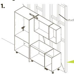
**Caution:** Please ensure all cabinets are screwed into your timber stud wall using a minimum of 65mm timber screws. If attaching to concrete, brick, steel or any other substrates seek advice from your hardware specialist.
