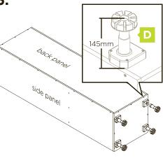
Set height of the adjustable feet to 145mm.
