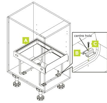
Align the bin frame (A) and the brackets (B) with the pre-drilled holes as pictured above and fix through the centre hole to the cabinet using 4x25mm wood screws (C).
