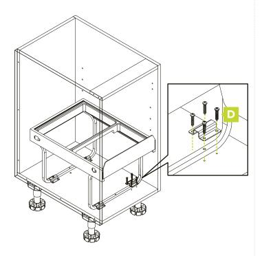
Further secure the bin frame and the brackets to the cabinet using 16 X 16mm wood screws (D) as pictured above.
