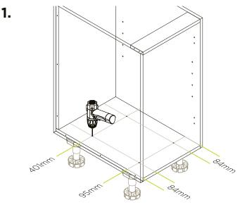
On the base of the cabinet mark out a line 84mm from the inside edge of the cabinet on both sides and then 95mm and 401mm back from the front edge of the cabinet as pictured above. Note: mesurements based on 400mm cabinet. Mark out all four holes to be pre-drilled where the lines cross.
