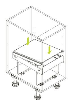
Slide the two back catches of the bin lid into the supports at the back of the frame. The two small front catches should now fit into the front supports.
