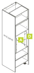
Attach the oven cleats 20mm back from the front of the end panels.
