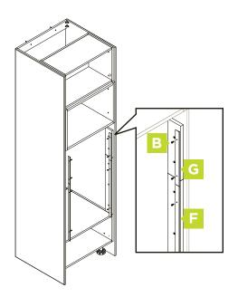
Attach both heat deflectors onto the sides of the end panels in front of the cleats.
