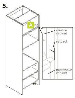
Attach the slimline cabinet on top of the mircowave box.
