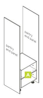
Set the drawer cabinet back from the front of the end panels 18mm for melamine doors and 20mm for thermoformed doors.
