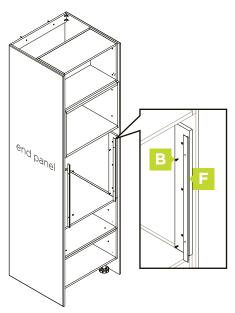
Attach the heat deflectors onto the sides of the end panels in front of the cleats.
