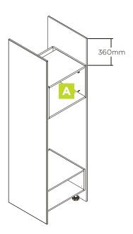
Attach the 600mm mircowave box 360mm from the top of the end panels.
