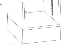
Pre-drill fixing holes as per marked positions using 2.5mm drill bit.
