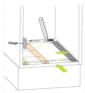
Place template in base of cabinet with dark grey bracket sitting opposite side to cabinet hinges. Mark drilling positions as per corresponding cabinet width.
