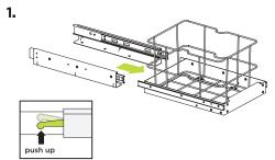
Separate runners from basket assembly using runner clips.
