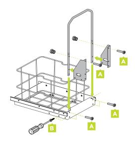
Attach handle to basket assembly using handle arms, nuts and bolts and screws.
