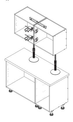
With the aid of cabinet supports align cabinets and hold together using clamps.
