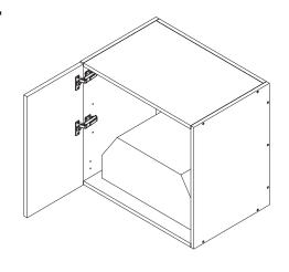
This cabinet can be installed with 2 x 300 medium wall cabinet doors for standard use, or 2 x 300 medium rangehood doors if required for an undermount rangehood.
