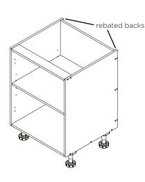
Base cabinets have been designed with the ability to assemble your back panel to create a 16mm rebate. The rebated panels can be trimmed down to accommodate uneven walls.
