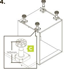
Set height of the adjustable feet to 145mm.
