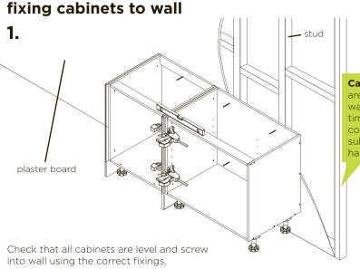
Caution: Please ensure all cabinets are screwed into your timber stud wall using a minimum of 65mm timber screws. If attaching to concrete, brick, steel or any other substrates seek advice from your hardware specialist.
