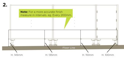
For uneven floors take the measurement from the floor to the bottom of the cabinet.
