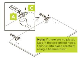
**Note:** install 2 more screws per carcase hinge plate (i.e.: a total of 4 screws) in round holes once the hinge has been adjusted!
