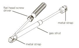
**note:** the gas strut can be adjusted by moving the bracket on the door forwards or backwards.
