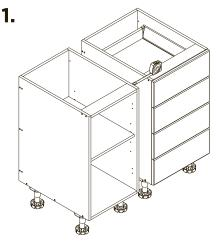
Measure the distance between the cabinet or wall where the filler panel will be installed.
