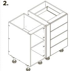
Attach the filler panel to the cabinet by predrilling and screwing through the cabinet into the offcut piece of timber.
