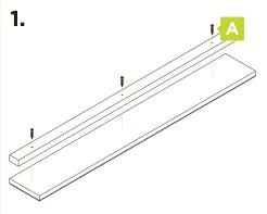
Attach either the off cut of the filler panel or a piece of timber to the back of the panel.
