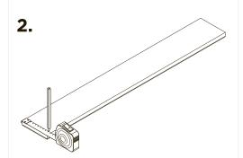
Transfer these measurements on to the filler panel and cut using a fine tooth circular saw or jigsaw.
