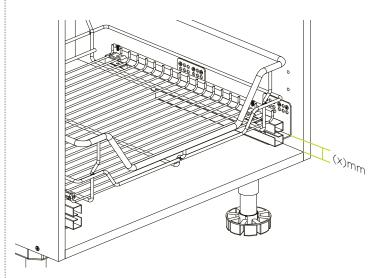
Measure from the base of the cabinet to the bottom of the basket runners (x).
