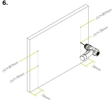
On the inside of your cabinet door or pot drawer panel, mark out and pre-drill four holes as per the diagram above, using measurement (x) from step 5. Use a 2mm drill bit to pre-drill holes to a depth of roughly 2.5mm.
