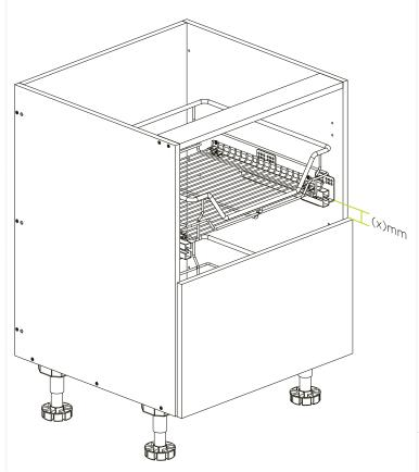
When installing a second pot drawer panel, measure from the top of the bottom pot drawer panel to the bottom of the runner to get (x).
