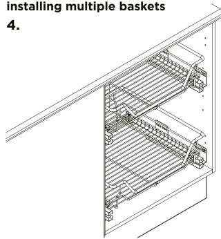
If you are installing multiple baskets in the same cabinet or pantry, repeat steps 1-3 ensuring you leave enough clearance between the baskets to accommodate the desired items. **Note:** If you intend to use the door mount hardware to attach a cabinet door or pot drawer panel, take into consideration their size, weight and positioning as well (see steps 5-11). The maximum weight capacity for the basket includes the weight of the cabinet door or pot drawer panel if installed.
