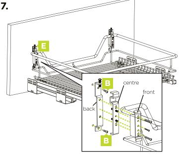
Disassemble the door mount hardware (E), as per the diagram above, by removing the three screws from the front piece.
