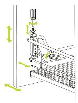
If required, adjust the height of door by tightening or loosening the top screw. Adjust the angle of the door by tightening or loosening the screws on the front piece. **Note:** To adjust the door panel left or right, loosen screws on the door mount hardware front piece, slide along the basket to desired position and re-tighten all screws.
