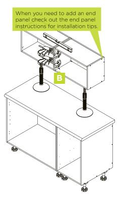
Check all cabinets are level then pre-drill and screw cabinets together.
