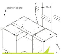
Caution: Please ensure all cabinets are screwed into your timber stud wall using a minimum of 65mm timber screws. If attaching to concrete, brick, steel or any other substrates seek advice from your hardware specialist.
