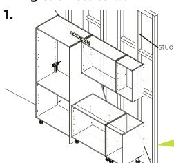
**Caution:** Please ensure all cabinets are screwed into your timber stud wall using a minimum of 65mm timber screws. If attaching to concrete, brick, steel or any other substrates seek advice from your hardware specialist.
