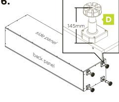
Set height of the adjustable feet to 145mm.
