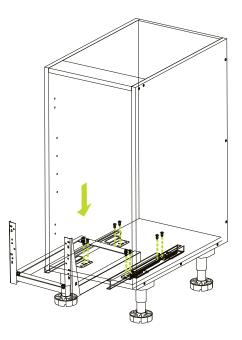
Secure the runners to the cabinet using a further  $8 \times 16$ mm wood screws, ensuring the screws are spaced evenly on both runners and are mirrored from the left to right side.
