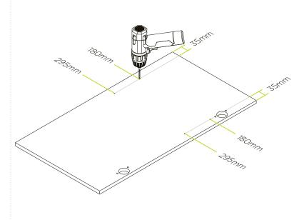
On the inside of your cabinet door, mark out and pre-drill four holes, measuring from the bottom of the door, as pictured above. Use a 2mm drill bit to pre-drill holes to a depth of roughly 2.5mm.
