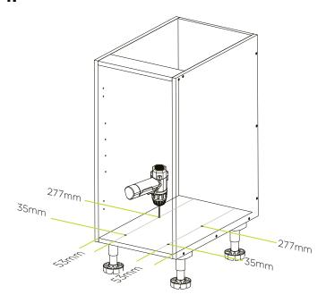
Mark out and pre-drill four holes on the cabinet base panel as pictured above. Use a 2mm drill bit to pre-drill holes to a depth of roughly 2.5mm.
