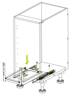
Align the runners with the pre-drilled holes and using 4 x 16mm wood screws (A), fix the runners to the cabinet. **NOTE:** Start with the second holes from the front of the runners to align with the pre-drilled holes.
