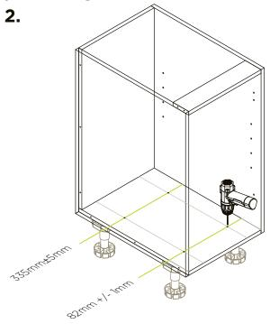
Pre-drill a hole, using a 2mm drill bit to a depth of roughly 2.5mm, where the lines cross.
