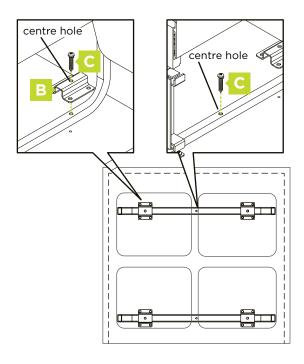
Align the bin frame (A) and the brackets (B) with the pre-drilled holes as pictured above and fix through the centre hole to the cabinet using 6x25mm wood screws (C).
