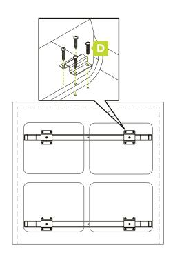
Further secure the bin frame and the brackets to the cabinet using 16 X 16mm wood screws (D) as pictured above.
