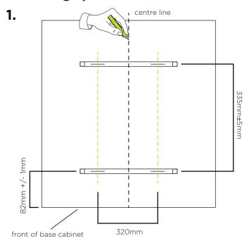
On the base of the cabinet mark out a parallel line in the middle of the cabinet. Then mark out 160mm from the centre line both ways. Lastly, mark out a line 97mm from the front edge of the cabinet as pictured above.
